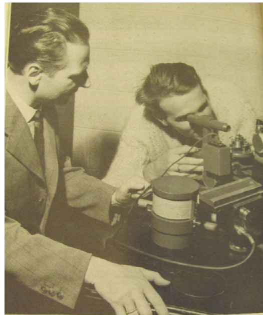
X-ray diffraction apparatus is used by metallurgical research team in the search for new compounds. Prof. Hans Stadelmaier is at the left (1964 Summary Brochure).
